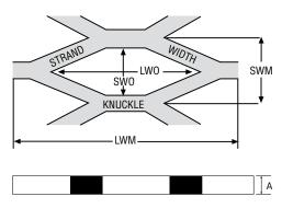
"A" Overall thickness and strand thickness
