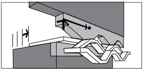
The upper knife ascends again, indexing (LWD) to its original starting position. The cycle continues until the sheet of expanded metal is complete.
